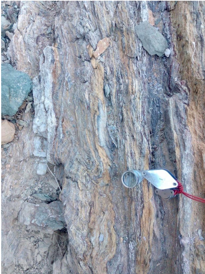
Figure 16. Pervasive silicification of shear zone with quartz veining – sampling target
