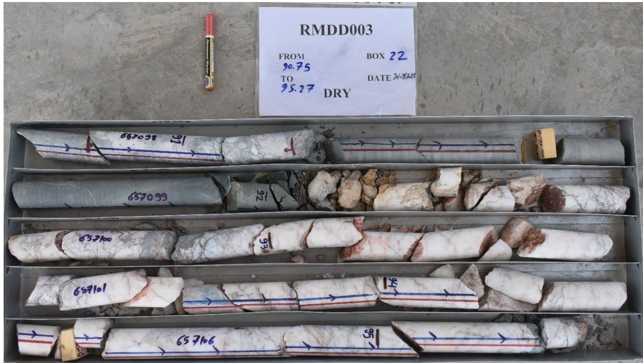
Figure 20. Example of core photography – Quartz vein in drill hole RMDD003.
