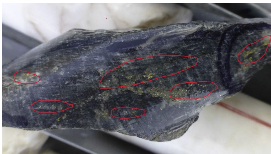
Figure 23. Visible Gold Grains DDH RMDD002
