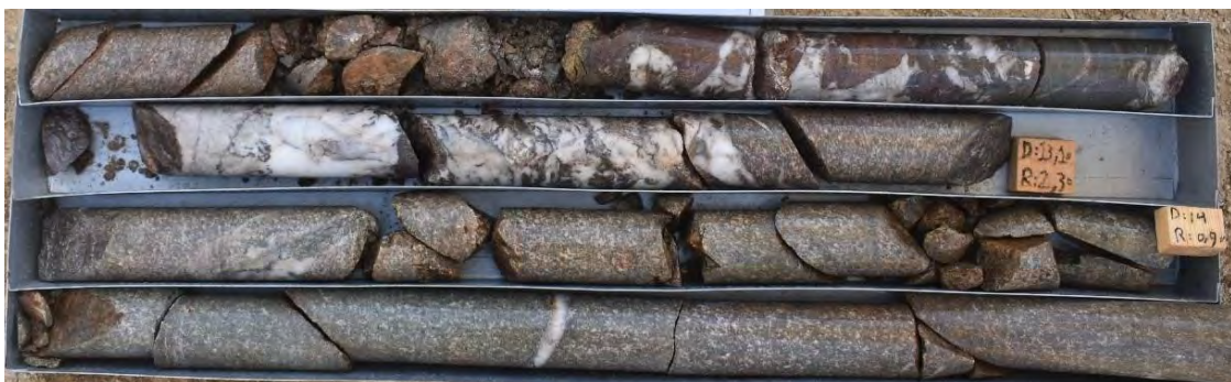
Fig. 2. showing brecciation quartz with carbonate alteration zone.
