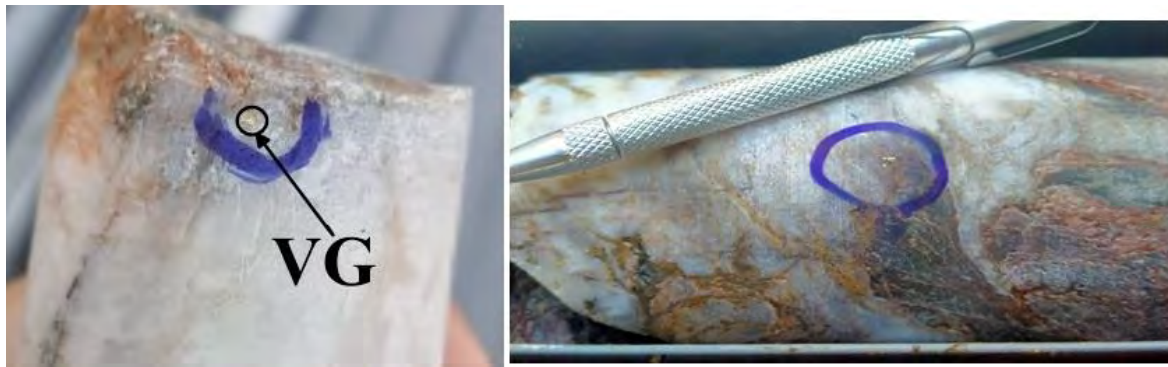
Fig.2 Core sample from borehole No. RMDD012 contain spots of visible gold (VG).
