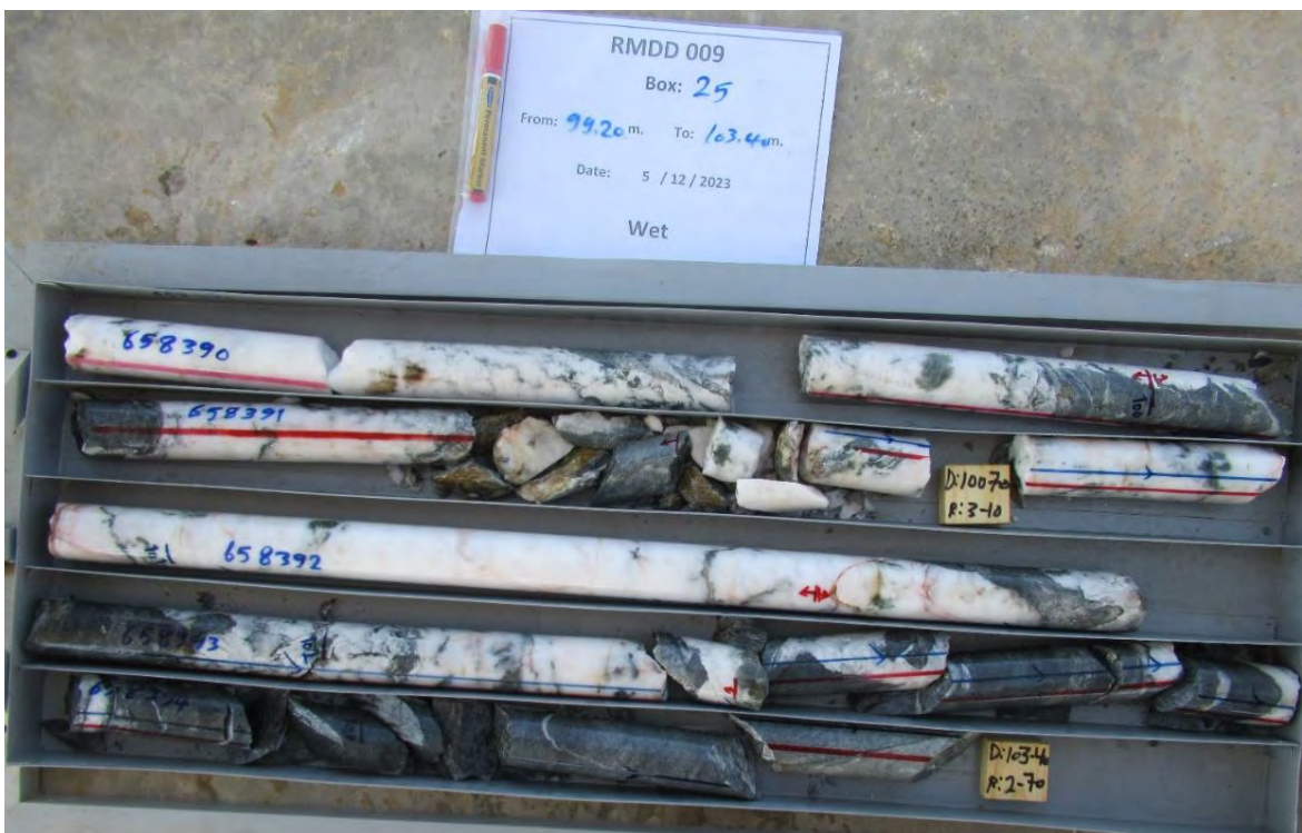
Fig. 2. Showing brecciated and white mineralized quartz vein.
