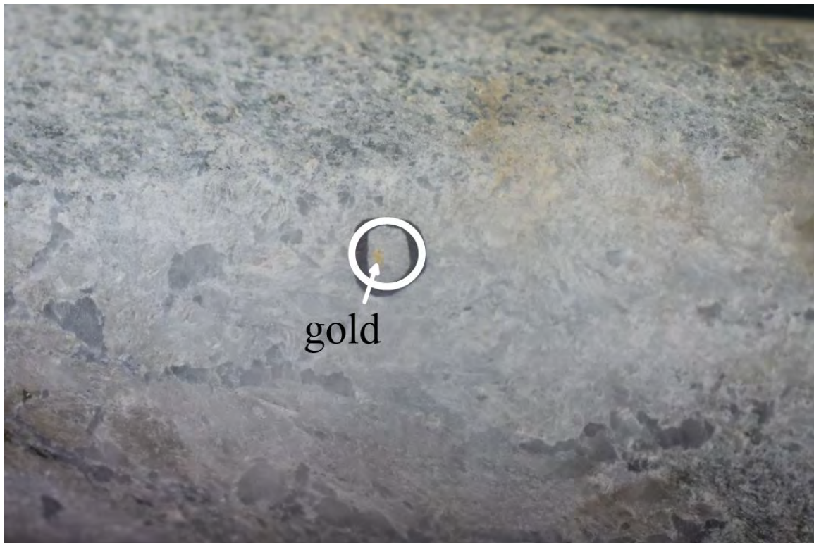
Fig.1. Fine disseminated gold in at the contact between quartz vein and quartz diorite.
