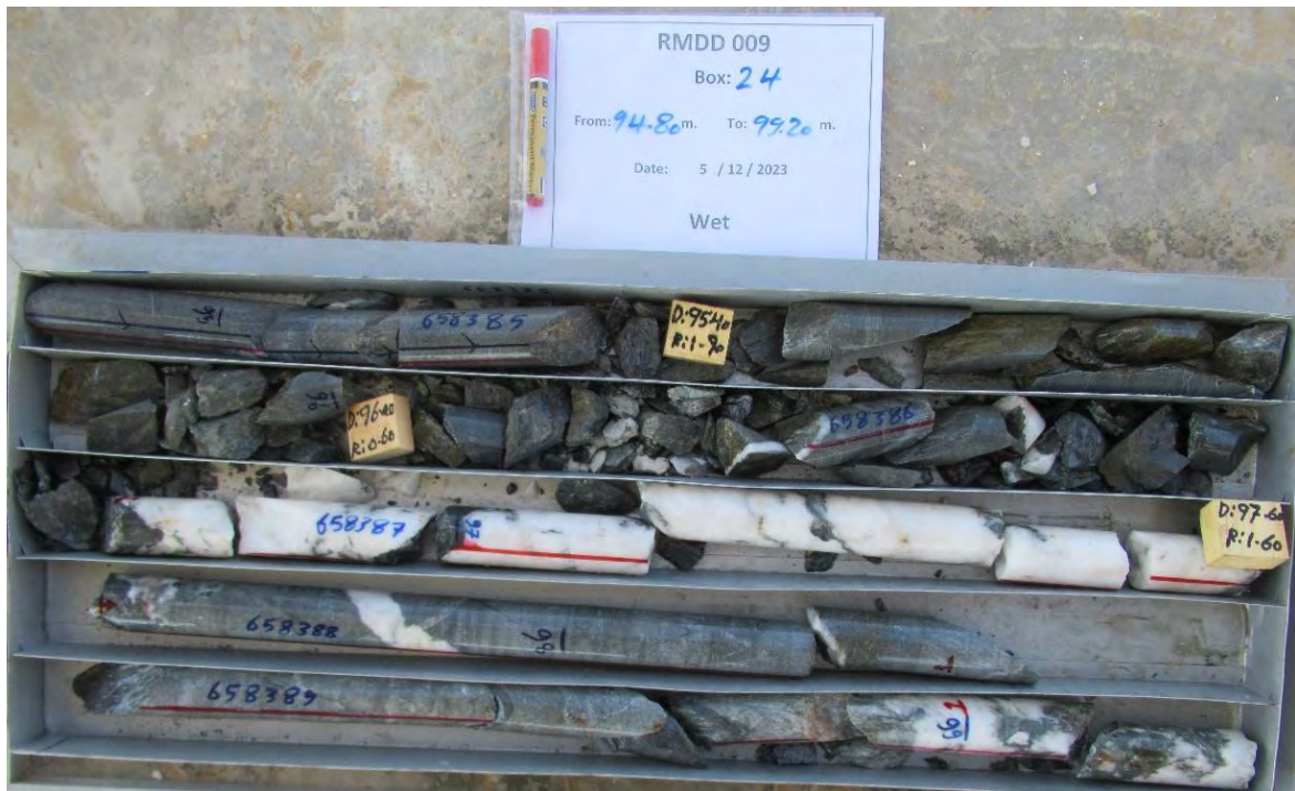
Fig. 1. Showing brecciated and white mineralized quartz vein.
