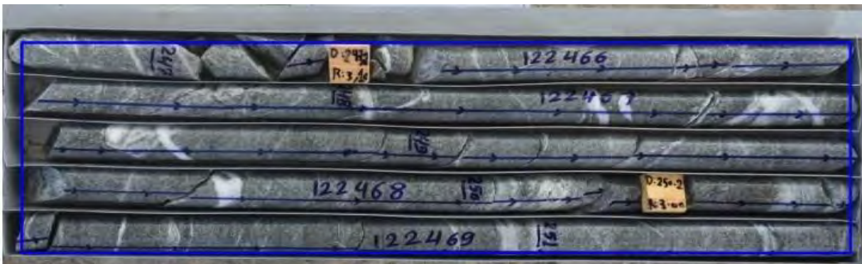
Fig. 4. Showing mafic dyke contact with quartz diorite.
