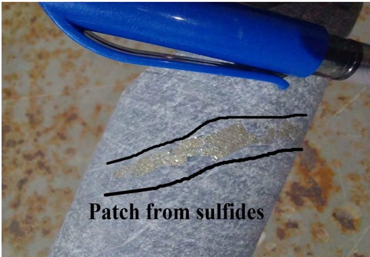
Fig. 4. Showing sheared quartz diorite intruded by patch from sulfides vein.
