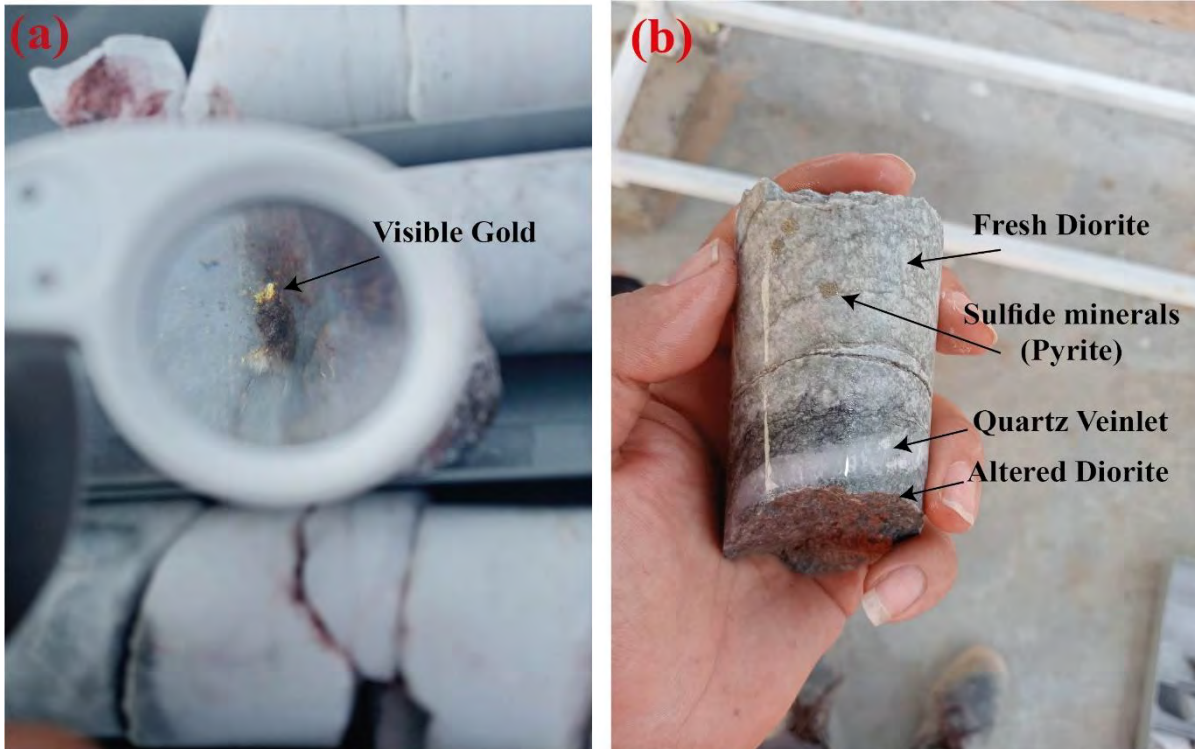
Fig.1. showing core samples; a) shows visible gold in quartz vein @ meter 127.1, b) shows the contact between fresh diorite and sheared diorite and fresh disseminated sulfides.
