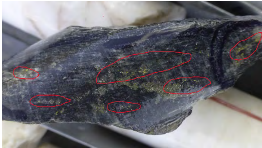
Figure 22. Visible Gold Grains DDH RMDD002
