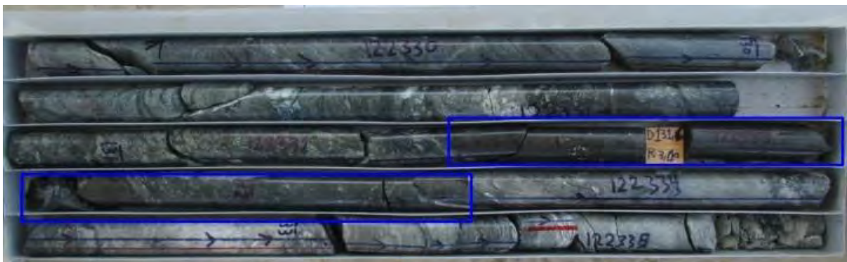
Fig. 4. Showing mafic dyke contact with quartz diorite.
