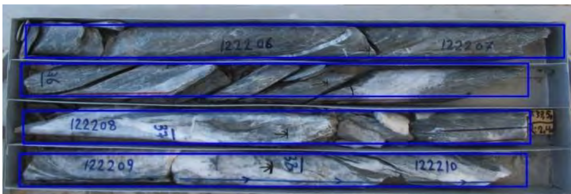
Fig. 2. Showing brecciation quartz vein.
