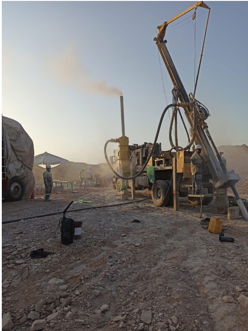
Figure 5. Reverse Circulation Drill Rig on site at Romeit
