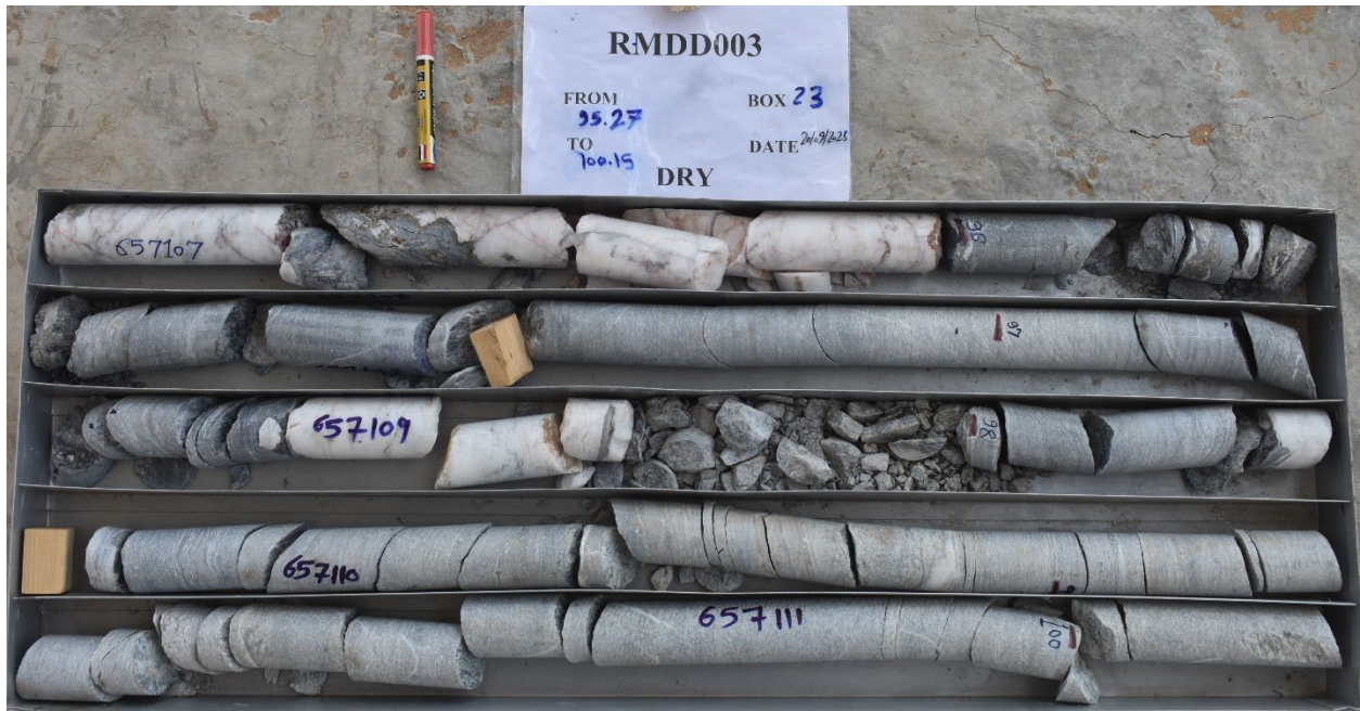
Figure 19. Example of core photography – quartz vein in drill hole RMDD003.
